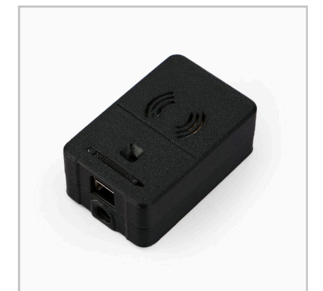
mmWave breathing Sensor [B.2]
